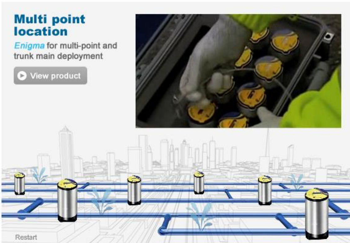
Figure 8-7 : Acoustic noise loggers/correlators (Source: Primayer)
